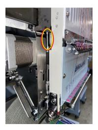
4. Needle Bars (springs behind take up levers)-1 drop on each needle bar spring weekly
